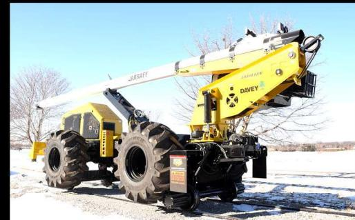
Discover the cutting-edge innovation of Mitchell Rail Gear Friction Drive Hi-Rail system, designed specifically for Jarraff Tree Trimmers. This remarkable technology transforms these machines into versatile dual-purpose machines capable of seamlessly transitioning between conventional Jarraff on-ground tree trimming to efficient on-rail tree trimming.
